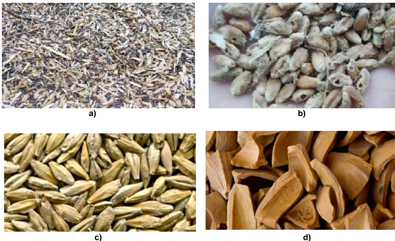
Figure 4 – Available types of raw material for activated carbon production in Kazakhstan: a) rapeseed waste; b) rotten, fungal-infected wheat; c) unripe rotten barley; d) shell of apricot kernels.
