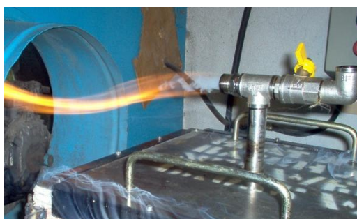
Figure 5 - Isolation and combustion of processing gaseous products of plant raw materials in the production of activated carbon.
