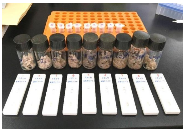
Fig. 10 -Test strips for clenbuterol, chloramphenicol and ractopamine
