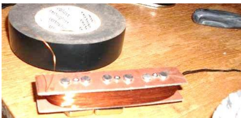
Picture 5. Pickup frame with inductance coil
