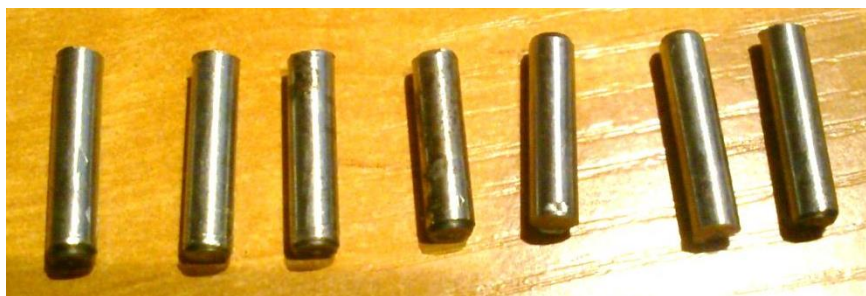
Picture 3. Steel cores for the pickup
