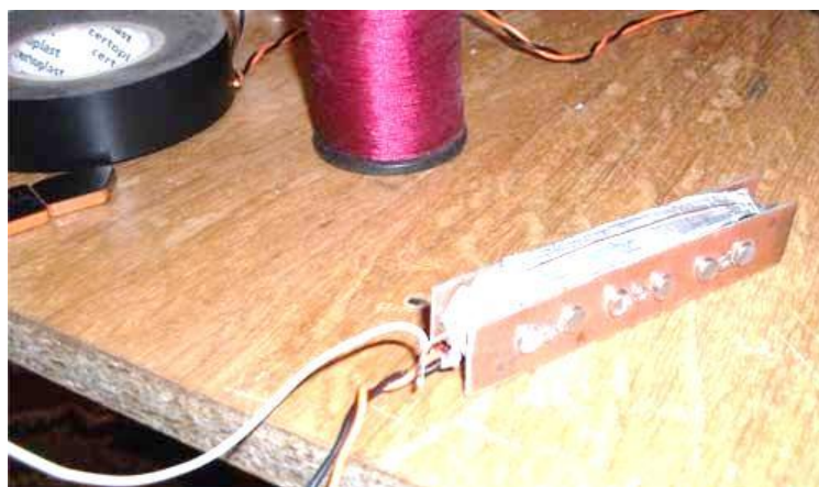
Picture 6. Coil shielding
